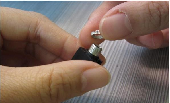
19. With the flat side of the 3D printed bear case **facing down**, insert the mono jacks to the corresponding paw or leg as depicted below. Insert the mono jack with the white wire with blue stripe to the right paw; blue wire to the left paw, white wire with orange stripe to the right leg, and the orange wire to the left leg.
