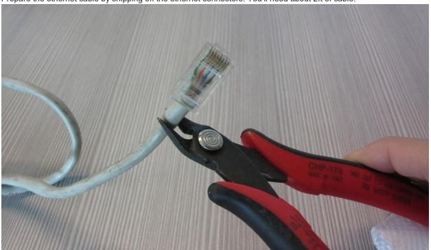
6. On one end, cut off the outer casing holding the 8 wires inside by 4cm and by 8cm on the opposite end.
